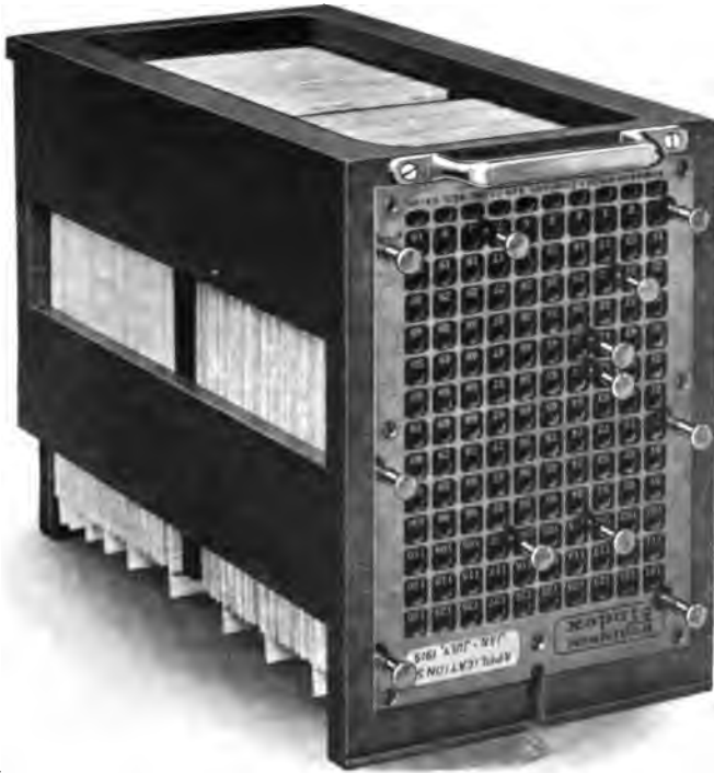
FIGURE 6. Index container in sorting position. This stage in the sorting process actually precedes the one illustrated in Figure 5. After the cards having the desired specifications have dropped down, a locking rod is inserted through the slot at the top of the inverted container. The locking rod passes through the short slot of the cards as shown at the top of Figures 3 and 4. In this illustration it has not yet been inserted. In Figure 5 the locking rod is shown in position.
